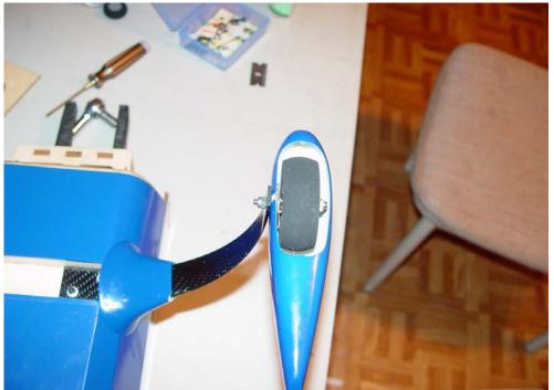
15. Next let's mount the tailwheel and rudder so we can get the Extra up on its feet, which will make the remainder of assembly much easier. Locate the rudder, 2 cut-down rudder horns and bases, tailwheel wire, aluminum mount, 2 coarse threaded wood screws, tailwheel and 2 small wheel collars.
