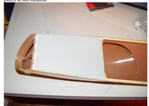
42. Use foam safe CA to secure the pilot and dash panel into position as shown. The dash panel should overhang the Depron floor by 1/8" to hide the seam of the 2 floor pieces.
