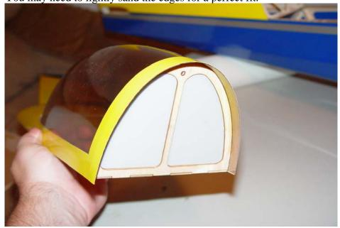
41. Hold the Depron canopy floor up to the bottom of the canopy/hatch and mark the location of the center of the cross member onto the Depron. Cut the floor into 2 pieces at this location.
