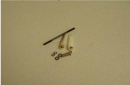
8. We highly recommend the use of the Dubro heavy duty control arm set for the Extra, Dubro part number 670 for Futaba, 671 for JR, and 672 for Hitec. For the aileron linkage we will use the 1.14" (28.9mm) arm. Electronically center the servo arm. Thread the ball links onto each end of the pushrod. Attach the pushrod to the servo arm and control horn using the supplied screws, nuts and
