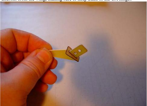
2. Use a sharp hobby knife to open the slot for the aileron control horn on the bottom of the surface. Insert the control horn into the base and into the slot in the aileron. Use a fine tipped felt marker to outline the base of the control horn.
