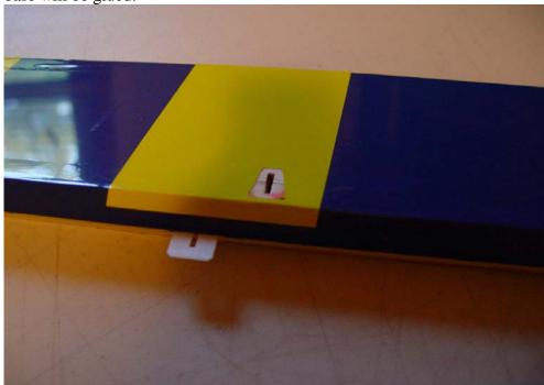
4. Scuff the part of the control horn that will be glued into the aileron slot with sandpaper. Mix up some 30 minute epoxy and apply to the slot and control horn and its base. Insert the control horn and base into the slot and push down until the horn is properly seated against the base and aileron surface. Wipe any excess epoxy away with a paper towel and some denatured alcohol.
