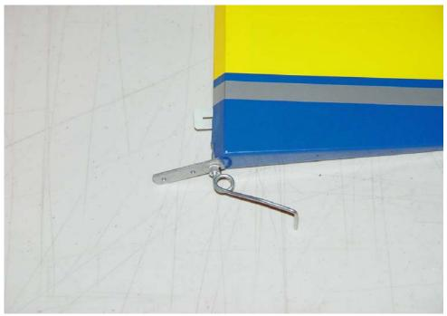
19. Slide the rudder into position on the rear of the fuselage and use thin CA to secure the rudder hinges.
