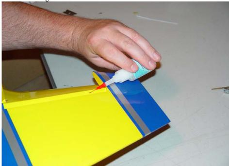
20. Align the aluminum mounting plate on the rear of the fuselage and secure with the 2 coarse threaded wood screws. You may want to wick a couple drops of CA into the mounting holes before final installation of the screws. Tighten the setscrew in the collar now.
