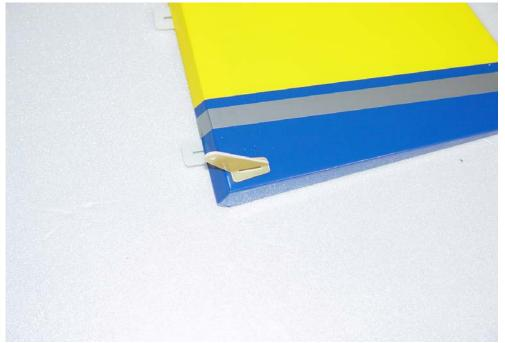
17. Slide one of the small wheel collars onto the landing gear wire and insert the wire into the aluminum mount. Use a pair of pliers to make a 90 degree bend in the wire as shown. Make sure to bend the wire so it is aligned with the rudder/fuselage. Wait to tighten the collar set screw until a later step.
