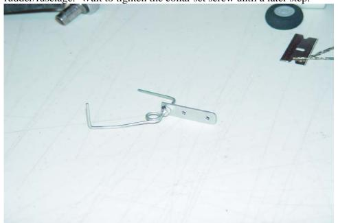
18. Drill a hole in the bottom portion of the rudder bevel to accept the tail gear wire and cut a slot from the hole to the bottom of the rudder to conceal the vertical portion of the wire. Glue the tailwheel assembly into the rudder with 30 minute epoxy. Be sure to coat the interior of the hole well with epoxy. You may want to add a piece of strapping tape over the wire for added strength. Place the tailwheel into position and retain with the remaining small wheel collar.
