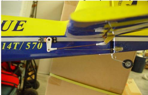
24. If using 2 elevator servos, use a razor saw to cut the hardwood elevator joiner flush with the edge of the elevator and glue this piece to the other side of the elevator to make the beveled portion complete. Then cut this piece flush with the side of the elevator. Use the same procedure as outlined above to install the 2<sup>nd</sup> servo, horn and linkage. You will need to join these two servos via a mix in your radio or with a reversing Y-harness.
