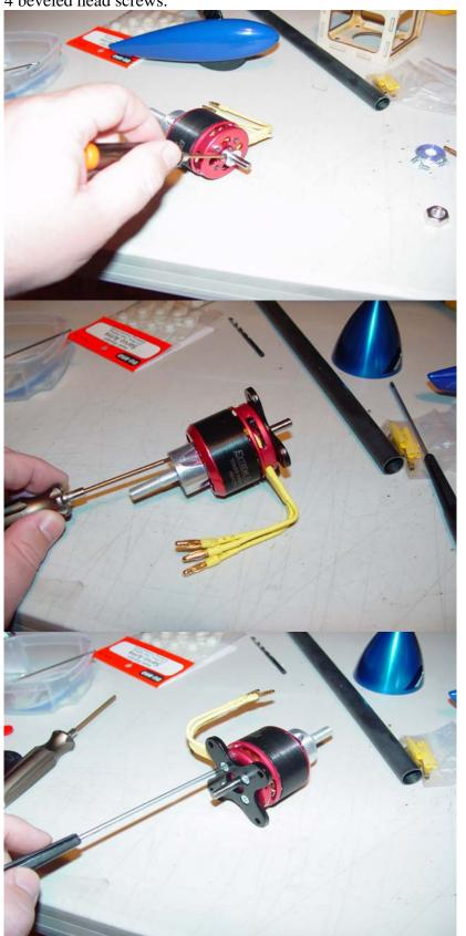
31. Next mount the motor to the front of the motor box using the remaining 4 bolts, washers and lock nuts. In the photos the motor is mounted before installing the motor box, but this is only for a better view of the mounting procedure. I have found it much easier to mount the motor box to the fuselage first, as outlined previously.
