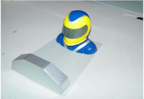
43. Slide the pilot/dash floor assembly into position through the portion of the canopy in front of the cross member. It may take a little effort, but is quite doable. Secure with foam safe CA. Slide the remaining piece of Depron floor into position and secure with foam safe CA. You may find installation easier if you cut off the front 3 or 4 inches of the Depron floor. This will be hidden under the canopy. See picture for detail.
