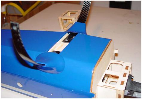
13. Glue the plywood mounting plate in the center of the wheel pant opening with 30 minute epoxy. Scuff the inside of the wheel pant with sandpaper before gluing. Once dry use a rotary tool to open a slot in the wheel pant using the slot in the ply plate as a guide. It should be big enough to slide over the threaded portion of the axle.
