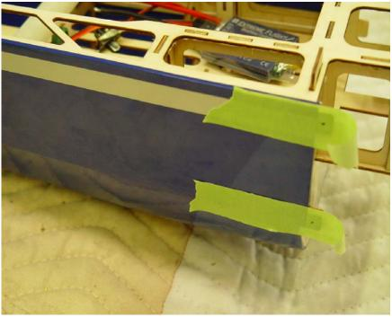
35. Place the canopy/hatch into position and secure with the spring loaded hatch latch. Peel the masking tape back far enough to place the cowl into position. Mount the spinner to the motor to aid in alignment. View the cowl from several perspectives to insure proper alignment and once satisfied lay the tape back into position on the cowl.
