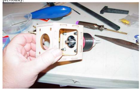
32. Mount the ESC in the position shown. You may want to add a scrap piece of balsa or lite ply here to facilitate mounting of the ESC. Use Velcro or cable ties to secure the ESC.
