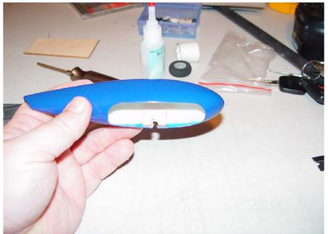
14. Place the wheel on the axle followed by the wheel collar. Slide the wheel pant over the axle with the retention ring inside the wheel pant. This ring will keep the wheel pant in place with friction. Insert the threaded portion of the axle into the hole in the end of the landing gear leg and secure with the nylon insert lock. Please see picture for detail.
