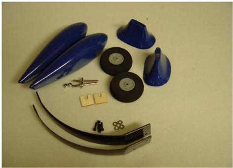
11. Before mounting the landing gear, take a minute to wick thin CA into all joints of the landing gear mounting area, both internal and external. Slide the 2 main landing gear legs into position from the side under the retaining lip. Secure the legs with the 4 3mm bolts, using a washer on each bolt. Be sure to use a drop or two of blue Loctite on each bolt.
