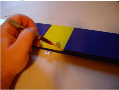
3. Remove the control horn and use your knife to remove the covering where the base will be glued.
