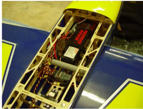
39. Insert the carbon fiber wing tube into the fiberglass socket and slide the wings into position and secure with the nylon thumb screws. The screw is inserted from inside the fuselage and into the blind nut in the wing root. Connect the aileron servo leads to the receiver. You may want to install 2 short servo leads into the aileron and auxiliary ports on the receiver to make plugging in the aileron servos easier. Alternately you can use a Y-harness for the aileron servos.
